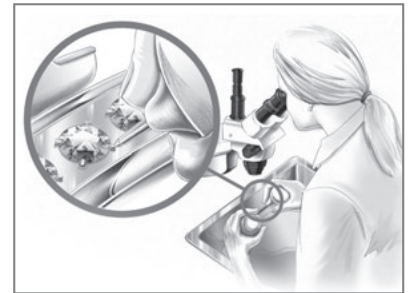
6 The manual beading and polishing of the prongs is often done under a microscope.
