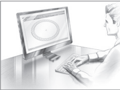
1 A CAD/CAM technical drawing of the stone-set part must be created first.
